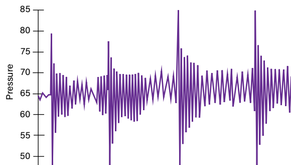
▲ Figure 1. This process plot shows pressure cycling in a stripping column.
