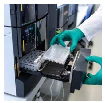
▲ Figure 3. An engineer from c-LEcta prepares an enzyme reaction in a 384-well microtiter plate for high-performance liquid chromatography (HPLC) analysis, which has become a standard tool for industrial enzyme development.
