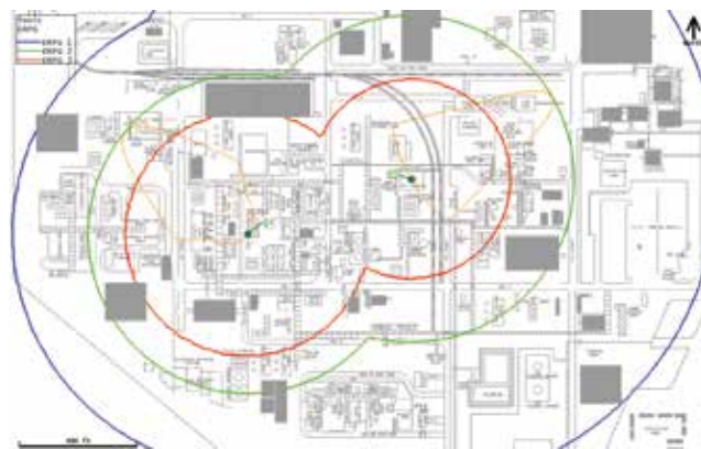
▲ Figure 2. Consequence modeling is used to evaluate the areas that an LOC incident could affect. The concentric circles represent areas with different projected levels of exposure. Personnel would experience mild effects within the blue area, serious effects within the green area, and life-threatening effects within the red area.
