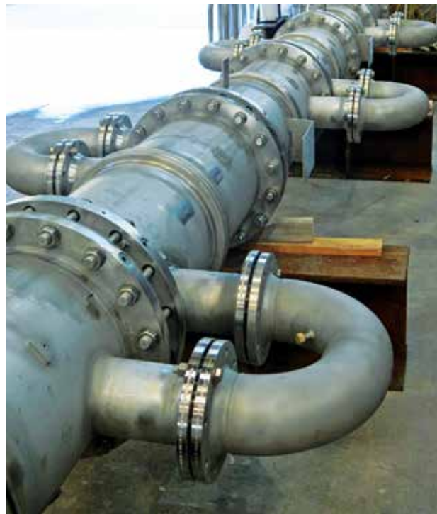
▲ Figure 3. This millichannel reactor is an example of PI in the spatial domain. Image courtesy of Ehrfeld Mikrotechnik GmbH.
