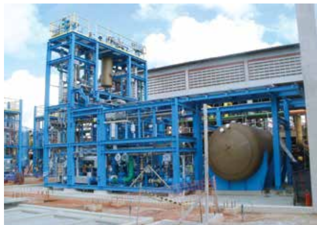
▲ Figure 2. This skid-mounted module is part of a chloralkali plant that can produce 15–45 ton/day of chlorine; a modular plant based on this design is being installed in Tanzania. Image courtesy of ThyssenKrupp Uhde Chlorine Engineers.
