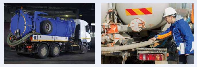
▲ Vacuum trucks are used to transport liquids, sludges, and slurries. Mixing incompatible materials or venting flammable materials near ignition sources can present fire and explosion hazards.
