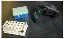
▲ A smartphone microscope can be used to detect norovirus in the field. Researchers have created a testing method, using a paper-based microfluidic chip, that enables simple counting of norovirus particles. Photo courtesy of Kristen Hanning, Univ. of Arizona Health Sciences.
