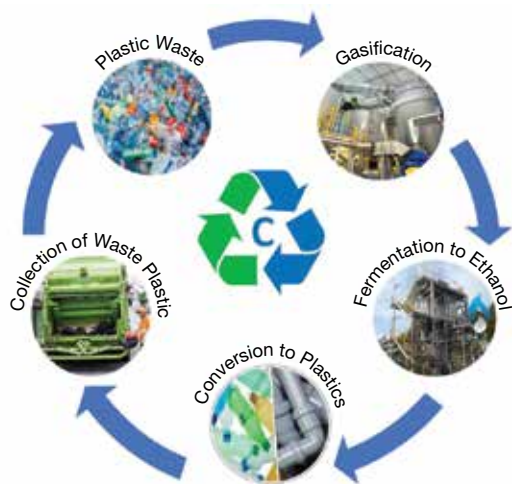
▲ Figure 1. Discarded products, such as unrecyclable waste plastic, can be broken down into building blocks, gasified, and transformed into valuable fuels and chemicals.
