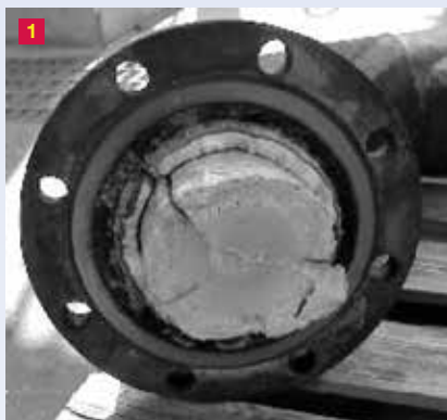
▲ Figure 1. In this particular incident, the vent line was obscured by layers of polymer.
