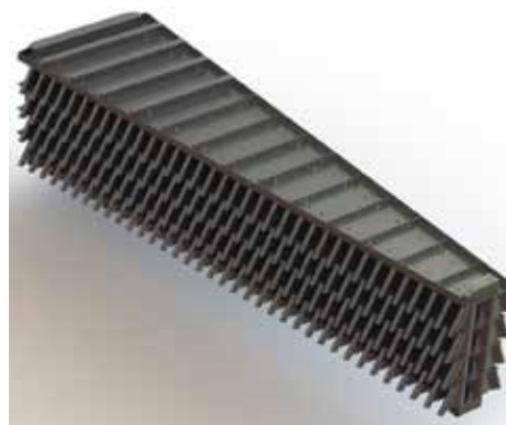
◀ Figure 4. Schoepentoeter-Plus is an advanced centrifugal device for deentrainment and vapor distribution commonly used for two-phase feeds into distillation columns. Figure courtesy of Sulzer Chemtech.
