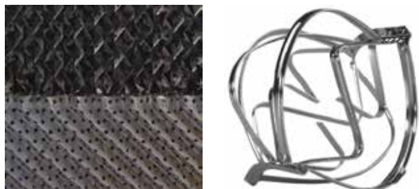
▲ Figure 6. FLEXIPAC HC (left) is a high-capacity structured packing and Intalox Ultra (right) is a high-capacity random packing. These designs attempt to enhance aerodynamics to reduce drag resistance in all directions of flow. Photos courtesy of Koch-Glitsch.
