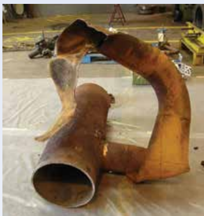
▲ Only after the insulation was removed were operators able to determine the cause of the failure to be external corrosion under insulation.
