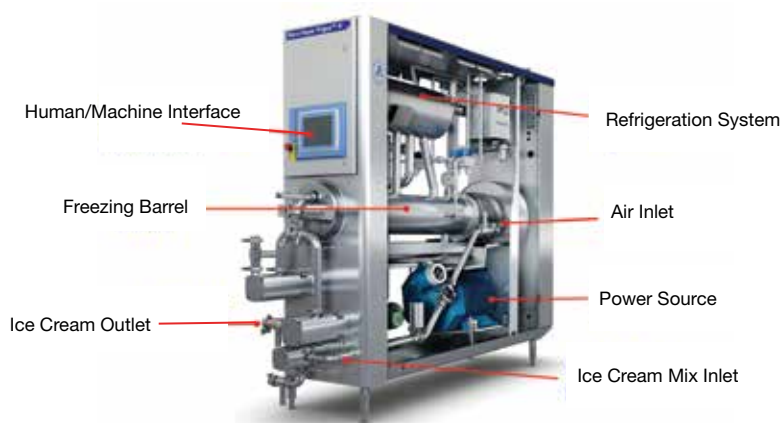
▲ Figure 2. This cutaway diagram reveals the interior of a modern ice cream freezer. Image courtesy of Tetra Pak.
