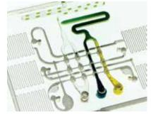
▲ This lab-on-a-chip is capable of autonomous mixing of fluids and compartmentalizing the resulting stream into individual droplets, which serve as miniature biochemical reaction vessels. Image courtesy of UCI (E. Werner, E. Hui).
