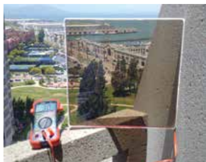
▲ The completed 1-ft 2 prototype LSC contains UbiQD's near-infrared quantum dots, which are laminated between two glass sheets.
