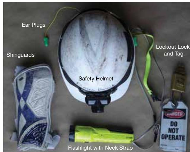
▲ Figure 5. I wear this safety equipment and bring my lockout lock and tag with me to all inspections.
