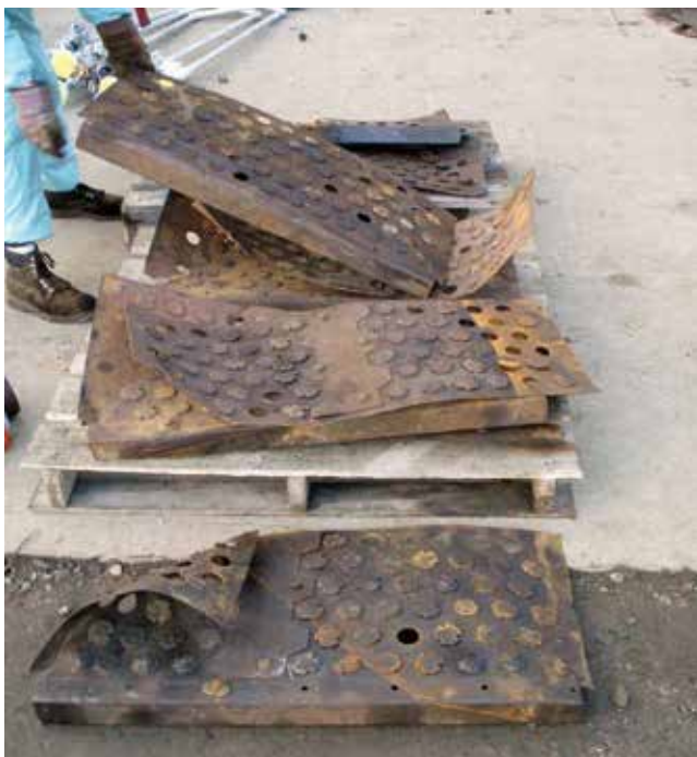
▲ Figure 21. Water hammer through high levels of liquid can push trays up.
