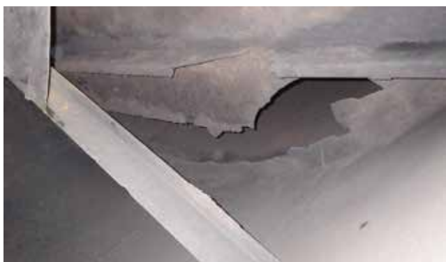
▲ Figure 8. You will need to decide whether cracked trays can be repaired or must be replaced.
