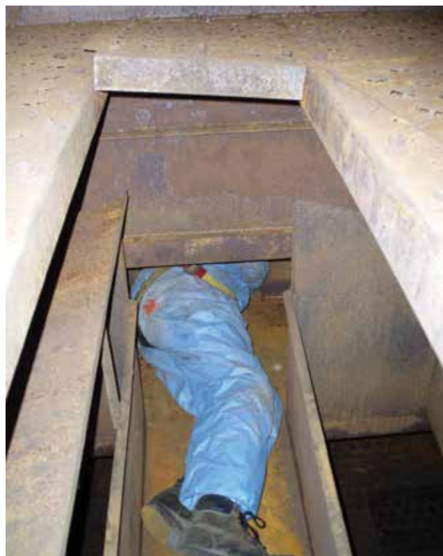
▲ Figure 3. You need a plan for safely entering and exiting a tight space. Body harnesses and other equipment can restrict movement.
