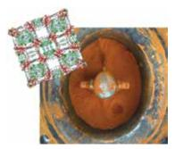
▲ framergy's 20-kg pilot ANG tank is loaded with AYRSORB F250 in preparation for wellhead flare gas capture from a live field slipstream in Texas. A digital rendering of adsorbed natural gas (green molecules) within AYRSORB F250 is also shown.
