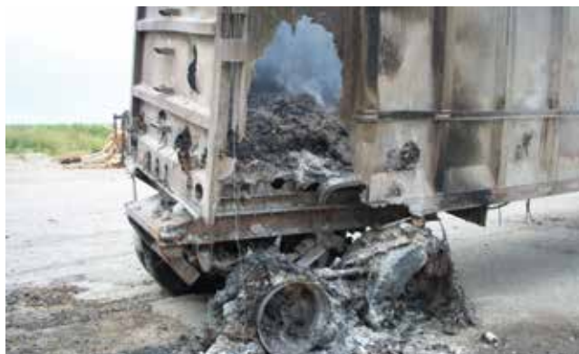
▲ Figure 8. The fire originated in the rear of the trailer, possibly due to overheated brakes.
