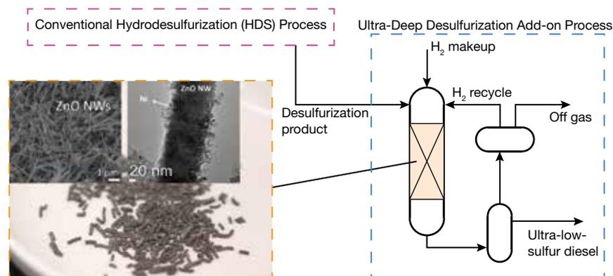
▲ Nickel nanoparticles are loaded onto zinc oxide (ZnO) nanowires to form catalytic adsorbents. Refineries can install a polishing step that uses these catalysts to reduce ultra-deep desulfurization costs and the environment impact of diesel production.
