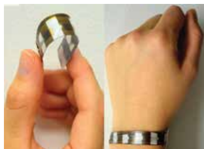
▲ A thin piece of cellulose paper containing 10 solar cells can withstand folding and bending (left), which makes it good for applications such as wearable devices (right).
