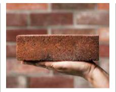
▲ bioMASON has developed a green process for growing bricks without the high temperatures typically used to fire bricks in kilns. At the core of the process are microbes that produce carbonate ions. The carbonate ions react with calcium ions to form calcium carbonate, which precipitates as biocement.
