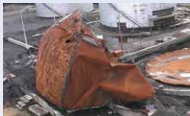
◀ Photo 1. A spark from hot work ignited vapors leaking from this spent sulfuric acid tank.
