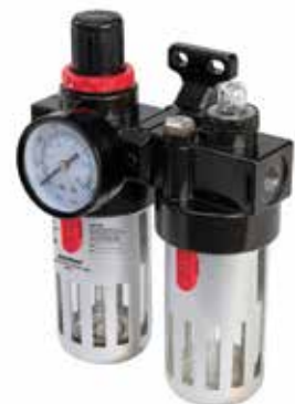
► Figure 7. The plastic bowls on the bottom of filter/regulator/lubricators (FRLs) are notorious for leaks. Establishing a formal air leak search, tag, and repair program can help document and remedy FRL leaks.
