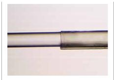
▲ Tetramer's polyimide coating (shown here on a fiber) can be stripped from fibers using a non-flammable, low-toxicity solvent. Conventional polyimides require hot sulfuric acid for removal.
