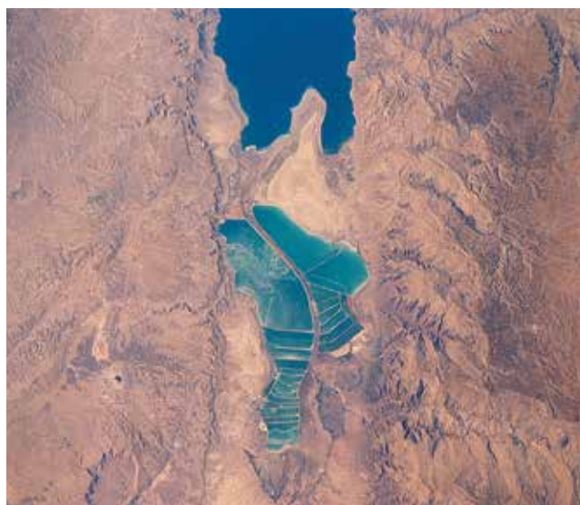
▲ Figure 2. Evaporation ponds at the south end of the Dead Sea enable extraction of potash and salt via solar energy. The eastern evaporation ponds belong to the Jordanian Dead Sea Works. Source: NASA Earth Observatory.
