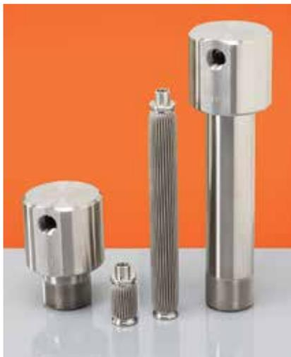
The FJV-3 Series high-pressure T-type filter assemblies feature all-stainless-steel construction for both the filter housing and filter elements. With working pressures up to 20,000 psi, these filters are intended for extreme environments, such as those found in offshore oil industry,
