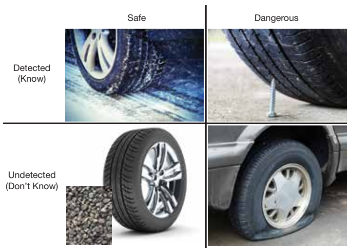
▲ Figure 4. Four types of failures are used to calculate the safe failure fraction. In a safe detected failure, a tire pressure sensor detects low pressure due to cold temperatures and alerts the driver. In a dangerous detected failure, a tire pressure sensor detects low pressure due to a screw puncture in the tire and alerts the driver of this dangerous condition. In a safe undetected failure, a rock embedded in a sensorless tire may cause a shift in pressure, but does not pose a hazard to the driver. In a dangerous undetected failure, a sensorless tire is flat and may cause the driver to lose control.
