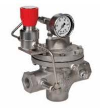
level required inside the cover dome to maintain the setpoint of the main valve. Because of its self-relieving feature, the SLR-1 is only appropriate for environmentally safe applications. The SLR-2 is similar to the SLR-1 in that it employs a P1/Fairchild regulator mounted onto a DA4 pressurereducing regulator. The SLR-2, however, is not self-relieving, which enables its use in hydrogen gas, natural gas, and sour gas applications. **Cashco, Inc.**
