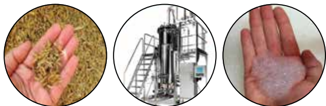
▲ Modular Genetics has used synthetic biology tools to engineer a Bacillus subtilis strain to convert cellulosic sugar via fermentation into an acyl glycinate surfactant, which can be used in personal care products such as shampoo.
