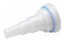
effective system minimizes chemical exposure during the transfer of chemicals from bulk containers to end-use applications. The 70-mm drum insert features a unique hybrid design that is compatible with both 70 mm  $\times$  6 mm and 70 mm  $\times$  5 mm thread forms. The connector features a robust seal below the threads, which allows it to be used in high-pressure applications. **Colder Products Co.** www.cpcworldwide.com
