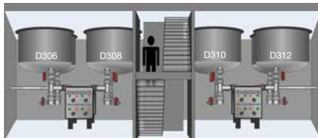
▲ Figure 7. Reactors D306 and D310 occupied the same place in their respective, identical tank rooms. At the bottom of the stairway, the operator became confused and went into the wrong room, where he emptied the wrong reactor. Source: (7).
