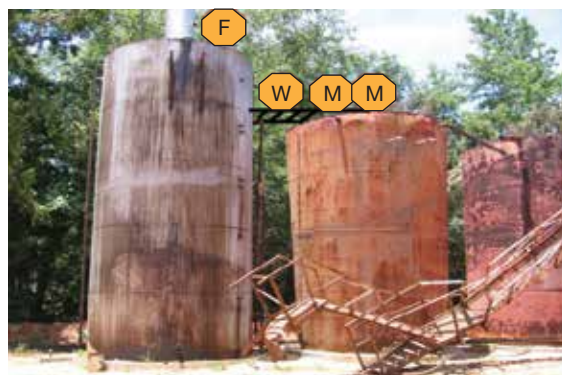
▲ Figure 5. The workers killed and injured in the Partridge-Raleigh oilfield tank explosion were on top of two tanks with a ladder stretching between them. The foreman (F) stood on Tank 4, while the two maintenance workers (M) stood on Tank 3, and the welder (W) positioned himself on the ladder. Source: (6).
