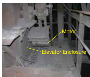
◀ Figure 8. Two workers went to inspect a bucket-elevator motor, which happened to be surrounded by piles of iron dust. During motor restart, vibrations dispersed powder on the floor and equipment. The dust ignited and created a flash fire, killing both workers. Source: (8).
