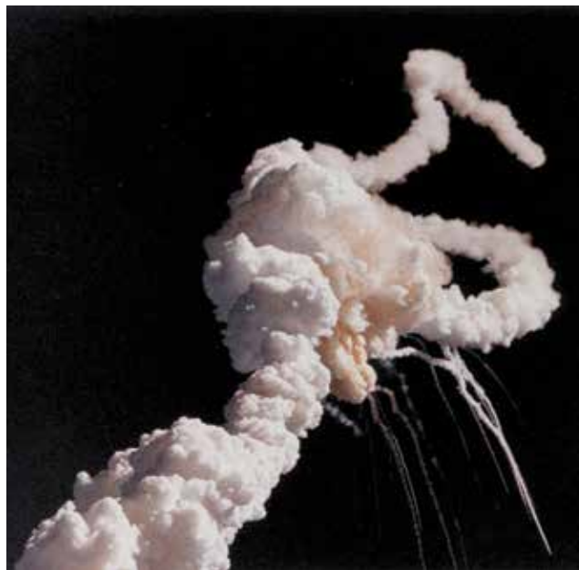
▲ Figure 2. On Jan. 28, 1986, the space shuttle Challenger and her seven-member crew were lost when a ruptured O-ring in the right solid rocket booster caused an explosion soon after launch. This photograph, taken a few seconds after the accident, shows the space shuttle main engines and solid rocket booster exhaust plumes entwined around a ball of gas from the external tank. Source: NASA.
