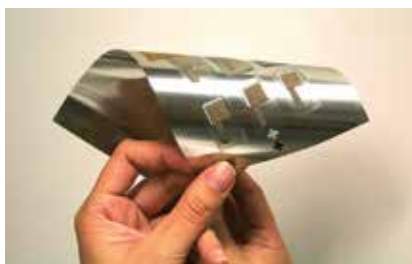
▲ Imprint Energy's ultrathin batteries (shown here printed on foil) offer high volumetric energy and power densities, rechargeability, low materials and manufacturing costs, inherent safety, printability, and form-factor flexibility that exceed those of any other commercial batteries with a thickness of <1 mm. Image courtesy of Imprint Energy.
