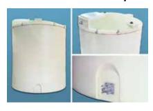
With a design capacity of 8,850 gal of liquid, the IMT 8850 double-wall storage tank can accommodate two truckloads of material. It features a standard 24-in. hinged manway opening, as well as a secure secondary containment sized for more than 110% of the primary tank capacity to reduce the likelihood of a chemical release, without the expense of lined. concrete containment. A heavy top
