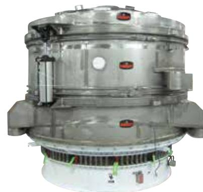
The K100-2(IRC)-SS round vibratory screener separates oversized particles from bulk materials at rates of up to 150 tons/hr. The screener includes a large, 75-ft<sup>2</sup> screening area and is totally enclosed for dust-tight operation. Above the conventional screen is a slightly smaller, high-capacity Cascade Internal Recycle screening deck comprised of two screens of the same mesh operating in series. This
