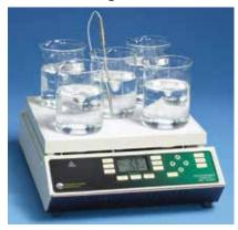
The EchoTherm Model HS65 programmable digital stirring hot plate has five stirring positions and can store up to ten programs with as many as ten steps each. Temperature, temperature ramp rate, stirring speed, and time can all be automated. The ceramic glass heating plate can be heated from ambient to 400°C, and is controlled to 1°C of the target.
