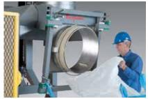
This ultraheavy-duty bulk-bag filling system combines the company's Swing-Down bulk-bag filler with a pallet dispenser and powered chain conveyor to provide a complete system that pelletizes and fills bags
