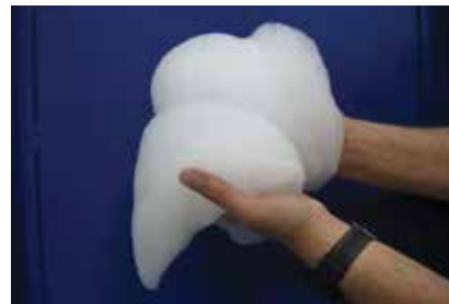
▲ Air and water mixed together to form a foam allows for rapid heat exchange. Image courtesy of SustainX.
