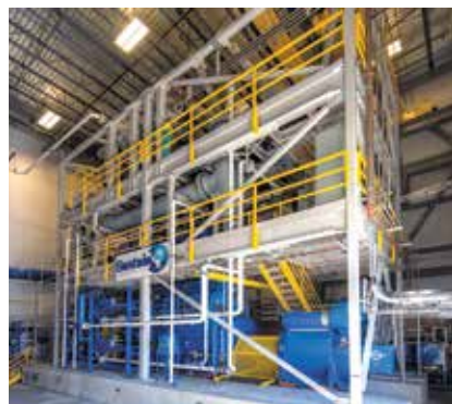
▲ SustainX operates a 1.5-MW ICAES prototype in Seabrook, NH. Image courtesy of SustainX.
