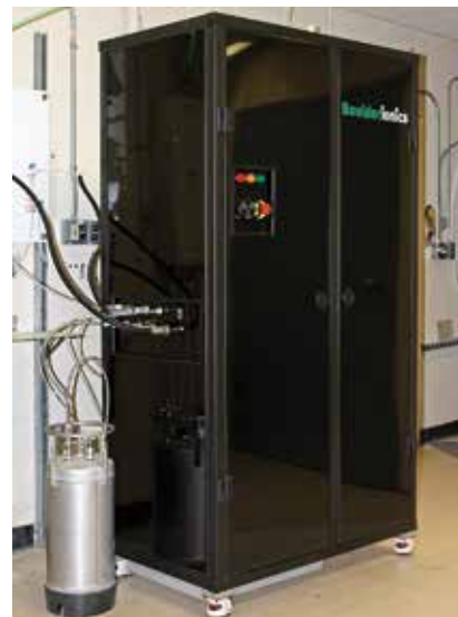
▲ Contained within this cabinet are arrays of tiny, microchannel and thin-film reactors that perform all of the steps for ionic liquid synthesis (alkylation, metathesis, separation, purification, and drying) in a continuous process. Image courtesy of Boulder Ionics Corp.
