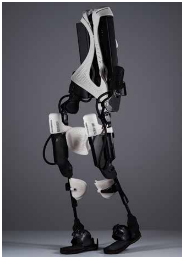
▲ Figure 5. A 3D-printed robotic suit has given a woman who was paralyzed from the waist down after a ski accident the ability to walk again. Debuted in February 2014 by 3D Systems, the robotic suit is the first of its kind. To construct the components, Valencia, CA-based 3D Systems obtained scans of the patient's thighs, shins, and spine, and then printed these using an SLS-type printer. The printed parts were then integrated with mechanical actuators and controls manufactured by Ekso Bionics. Image courtesy of 3D Systems.
