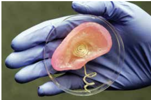
▲ Figure 6. Scientists at Princeton Univ. used a 3D printer to fabricate a bionic ear that was able to receive signals across a frequency spectrum of 1 MHz–5 GHz (beyond the 20 Hz to 20 kHz range of a human ear). Image courtesy of Michael McAlpine, Princeton Univ.
