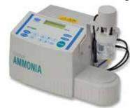
The AT-2000 ammonia analyzer measures ammonium-nitrogen (NH<sub>4</sub>-N) with a short measurement time of approximately one minute. It is easy to use, does not require specific operator training, and does not need to be calibrated prior to the sample run. It can measure small sample volumes of 0.1 mL, 1 mL, or 10 mL. The electrode is stain resistant and is not impacted by temperature changes.
