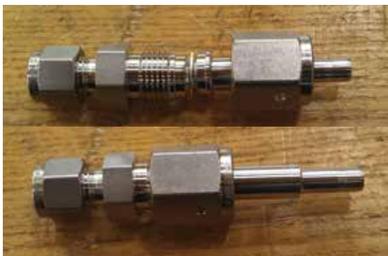
▲ Figure 10. This vacuum fitting has a metallic gasket. It is shown open (or disassembled) in the top photo, and closed (assembled) in the bottom photo.
