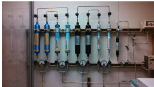
▲ Figure 14. Heavy equipment requires specialized mounting to minimize stress on the tubing.
