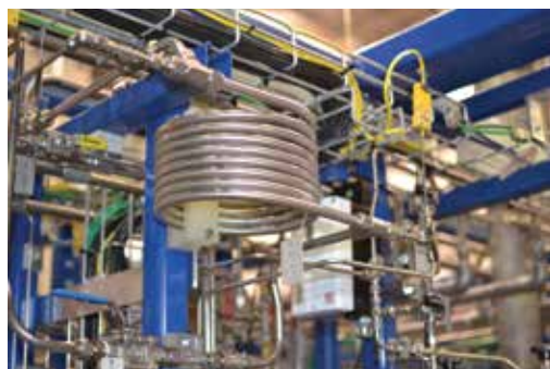
▲ Figure 6. Tubing and compression fittings are frequently used in pilot plants. Tubing is easy to install and can be bent, which allows for intricate shapes and specialized construction. Photo courtesy of Zeton, Inc.
