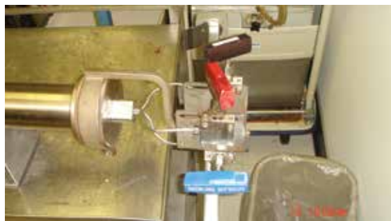
▲ Figure 13. Mounting the valves, instead of the tubing, can lower stress on tubing and prevent leaks.
