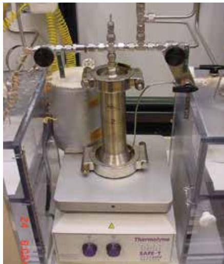
▲ Figure 12. Two sanitary fittings and a piece of piping are used to create a vessel.
