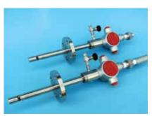
The FPT-850EL is now available in lengths up to 1.2 m with a diameter of 27 mm. The near-infrared transmission probe has been developed to provide maximum long-term reliability under the extreme conditions of high temperature, thermal shock, and aggressive chemistries. The probe is designed with a proprietary seal that guarantees that the only materials in contact with
