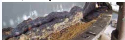
▲ Corrosion resulting from damaged insulation
