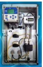
the pH, and drains and rinses the sample cell, discharging a sample with a safe pH near 8. The SMS-22 is a sequential sampling analyzer, with sample timing that is easily adjust-able from two samples per hour to 10 samples per hour. Its 4–20-mA output displays the total sulfide-ion content as well as the pH value. The rugged enclosure provides IP66 protection and is rated NEMA 4X.
