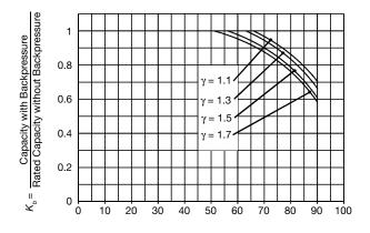
▲ Figure 7. Use this plot to determine the backpressure correction factor,  $K_b$ , for conventional spring-operated relief devices in vapor service. It is drawn using the equation and constants in Table 2 and data from Ref. 3.
