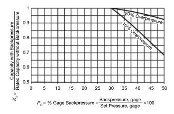
$\blacktriangle$  Figure 8. Use this plot to determine the backpressure correction factor,  $K_b$  for balanced-bellows relief devices in vapor service. It is drawn using the equation and constants in Table 3 and data from Ref. 3.
