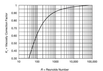
Figure 6. Use this diagram to determine the viscosity correction factor,  $K_{a}$  for both conventional and balanced-bellows relief valves in liquid service. The figure is drawn using the equation  $\ln K_v = 0.0857 0.9541/\ln R - 35.571/R$  and data from Ref. 3.
