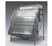
The Cross-Flo static dewatering sieve continuously removes solids from waste streams at ultrahigh rates, which facilitates clarification and dewatering of slurries. The screening deck is fitted with a stainless steel wire screen that has slots oriented perpendicular to the flow of material. An extended acceleration/orientation ramp in the upper por-
