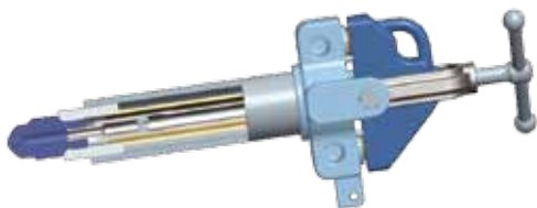
▲ Figure 9. This oil gun has a concentric tube design. Oil flows through the inner tube, while the atomizing medium, typically steam, flows through the annular area between the inner and outer tubes.
