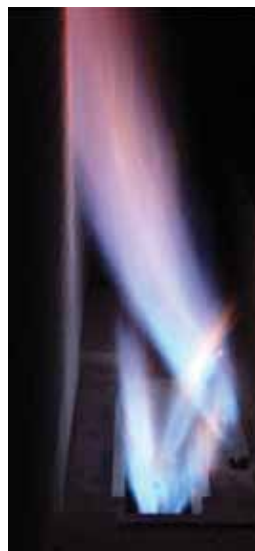
◀ Figure 4. This flat flame is produced by a wall-fired burner.
