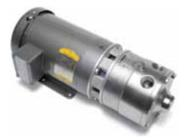
Because the stainless steel, magneticdrive Coro-Flo MDC pump has no mechanical seals, maintenance requirements are significantly reduced. Sealless technology offers maximum protection when handling corrosive and toxic chemicals, because it prevents emissions to the atmosphere. The pump has a close-coupled design that makes installation quick and easy. Its stainless steel construction is wellsuited for highly corrosive applications. **Corken, Inc.**
