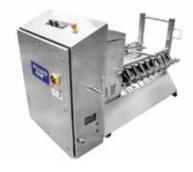
With a unique delivery system that improves coating results, this equipment can be custom-designed for a variety of tablet coating requirements. The system consists of a modular airatomizing manifold, a liquid-delivery skid, and Batch Arichitect process controls. The removable spray bar features anti-bearding nozzles, internal recirculating guns, a shutoff valve, and a mounting design that prevents tablet entrapment. The system has a custom programmable logic controller
