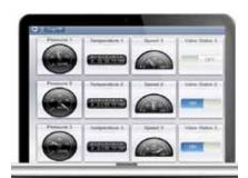
This SCADA/HMI visualization app offers mobile access to the company's Web Studio applications from any Windows 8 or Windows RT device. SCADA information can be accessed from a variety of mobile devices, such as phones, tablets, and laptops. The app allows users to monitor critical information — such as alarms, process values, trends, and historical data — at any time from any location via the Windows 8 operating system. The application is available at The Windows Store.
