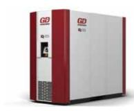
The IQ high-speed blower package includes a variable-frequency drive, permanent magnet motor, and a proprietary impeller design, all within a sound-dampening enclosure. The package's programmable logic controller (PLC) can be seamlessly integrated with existing plant operating systems. At its maximum operating speed, the blower delivers up to 10,000 ft<sup>3</sup>/min and up to 20 psi.
