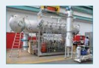
Unique research grade vacuum dryer capable of drying both solid feeds (powder and discrete pieces) and pumpable fluids. Diagram below shows three and single belt configurations for solid and fluid feeds respectively.
